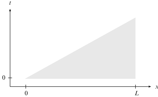
Fig. 9.1 Portion of the x - t plane (shaded region) in which the solution to (9.1) is determined by the initial data \psi(x, 0) , 0 \leq x \leq L
