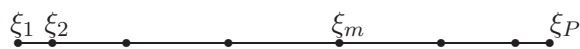
Figure 15.7: Distribution of collocation points in a spectral element. In this example there are 8 collocation points (polynomial of degree 7).
