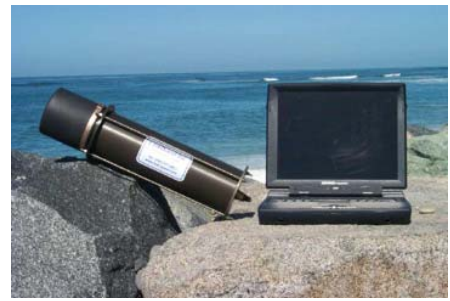
LinkQuest Underwater Acoustic Modem for M3A-E1 buoy in the Cretan Sea
