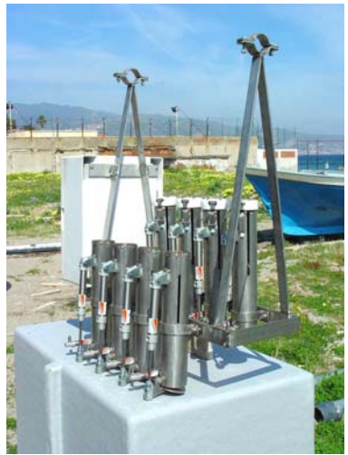
Development of a multiple launcher for expendable probes
