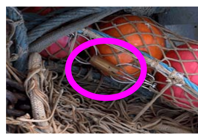
The Fishery Observing System - Real Time recording system: LOG-BOOK and temperature and pressure recorders installed on the net
