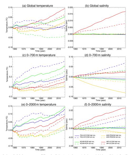
**Figure 4.** Time evolution of global temperature ( ${}^{\circ}$ C) and salinity (psu) change (relative to initial conditions) for all experiments (depth-integrated, upper 700 m, upper 2000 m).
