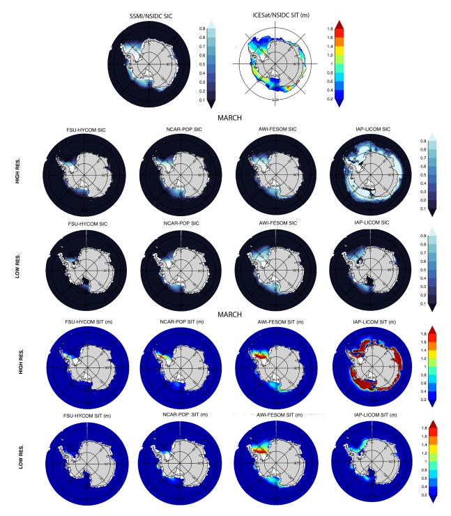
**Figure 32.** Southern Hemisphere summer mean (March) sea ice concentration (SIC) and thickness (SIT). Top panels: 1980–2018 SIC from passive microwave satellites and 2003–2007 SIT from ICESat. Lower panels: 1980–2018 modeled SIC and SIT.
