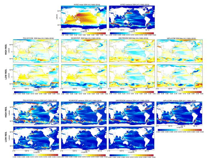
**Figure 17.** Top panels: mean 1993–2018 SSH and variance AVISO. Middle panels: difference between the mean modeled SSH and AVISO SSH. Bottom panels: modeled variance derived from 5 d average outputs. The low-resolution IAP-LICOM SSH variance was not provided.
