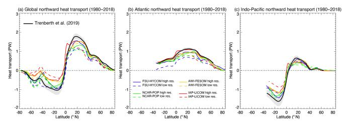
Figure 28. Modeled time mean meridional heat transport in PW over 1980–2018: (a) global, (b) Atlantic Ocean, and (c) Indo-Pacific Ocean. Black lines are the latest observational results from Trenberth et al. (2019) with uncertainties.
