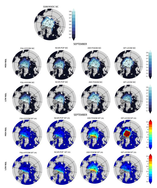
**Figure 30.** Northern Hemisphere summer mean (September) sea ice concentration (SIC) and thickness (SIT). Top panel: 1980–2018 SIC from passive microwave satellites (summer SIT not available from ICESat). Lower panels: 1980–2018 modeled SIC and SIT.
