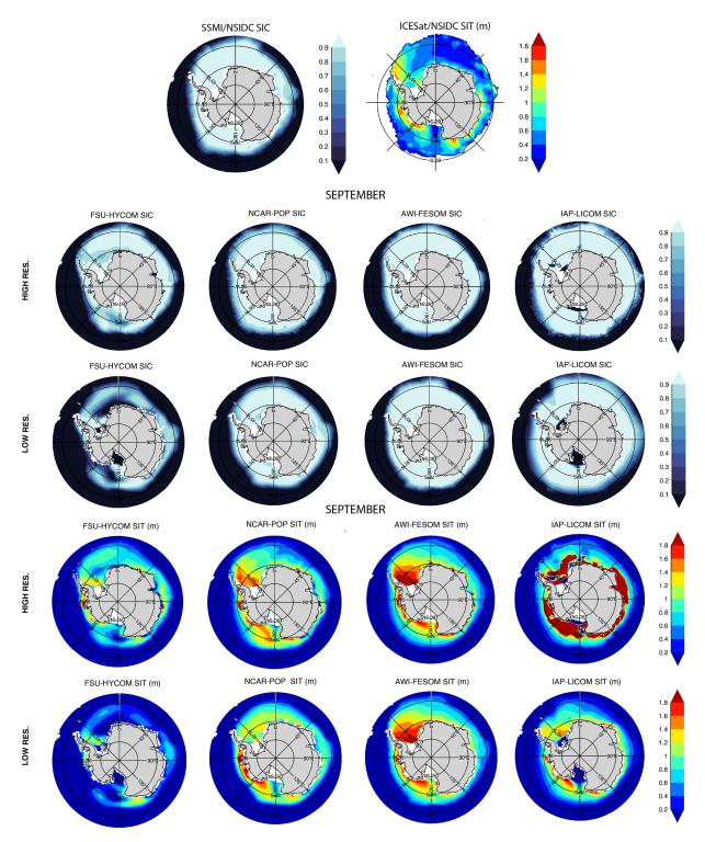
**Figure 31.** Southern Hemisphere winter mean (September) sea ice concentration (SIC) and thickness (SIT). Top panels: 1980–2018 SIC from passive microwave satellites and 2003–2007 SIT from ICESat. Lower panels: 1980–2018 modeled SIC and SIT.
