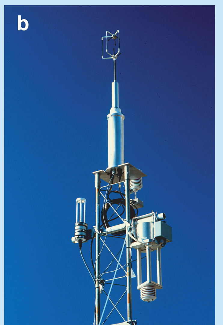
Figure 3: (a) R/V Roger Revelle and WHOI flux reference buoy. (b) ETL direct flux sensors. Photo credit: Chris Fairall.
