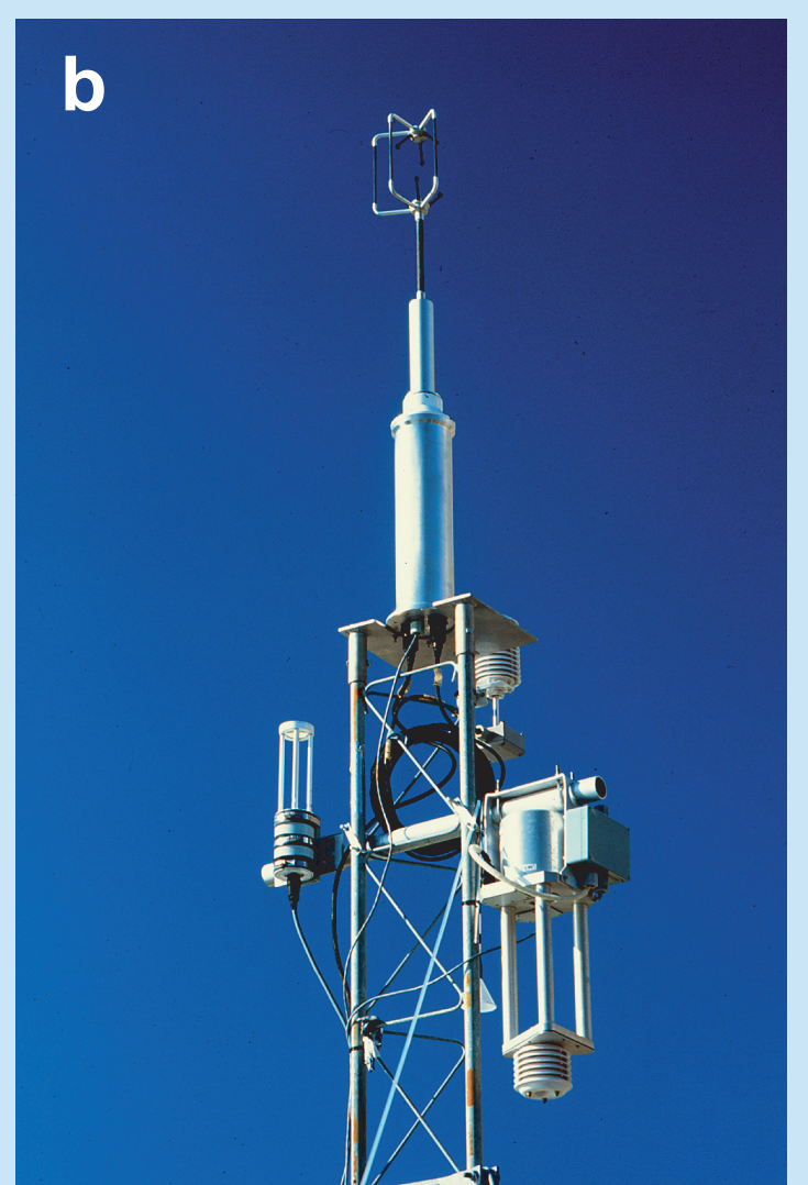
Figure 3: (a) R/V Roger Revelle and WHOI flux reference buoy. (b) ETL direct flux sensors. Photo credit: Chris Fairall.
